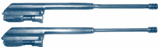
4. Bolt-it is used for placing the cartridge into the chamber of the gun, for closing the duct of the barrel when shooting, for producing a gunfire and for taking the shell out of the chamber.
