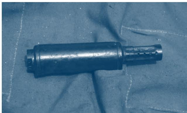
7. Gas chamber-gas chamber serve to direct the gunpowder gases from the barrel to the piston.
